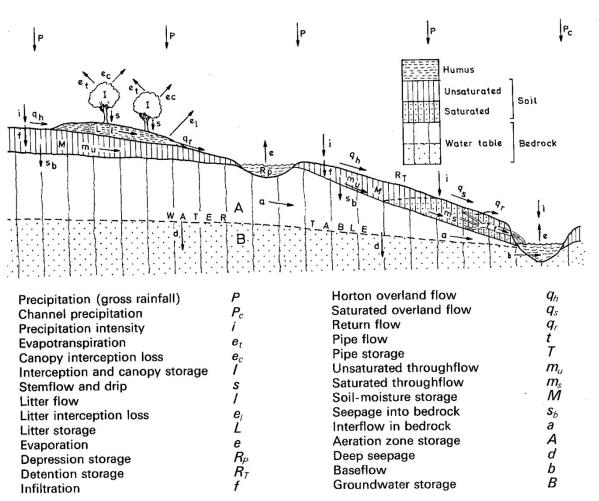
Figure 1.2 Components of the hillslone hydrological cycle
